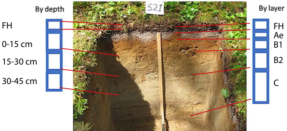
Fig. 1: Sampling by increment depth or by soil layer. Image from: https://www.nrcan.gc.ca/our-natural-resources/forests/sustainable-forest-management/conservation-and-protection-canadas-forests/soil/13205
