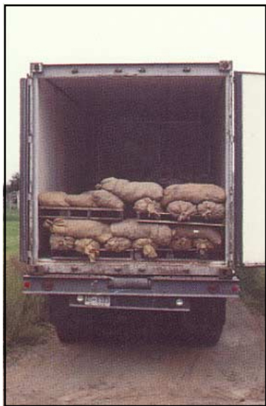
FIGURE 25. Loading of cones onto transport truck using pallets for spacing
