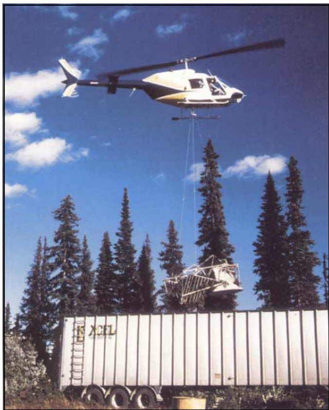
FIGURE 15. Helicopter dumping cones from aerial shear into a transport truck
