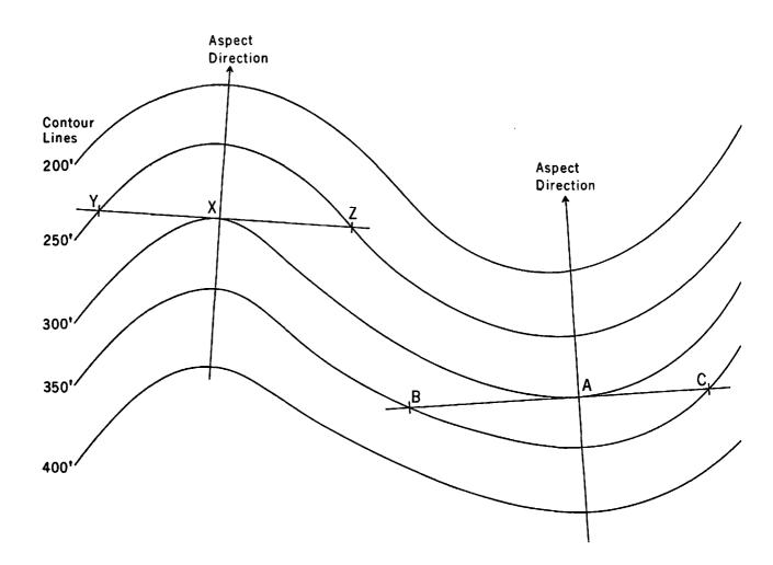
Fig. 4. MEASUREMENT OF SHAPE OF CONTOURS
