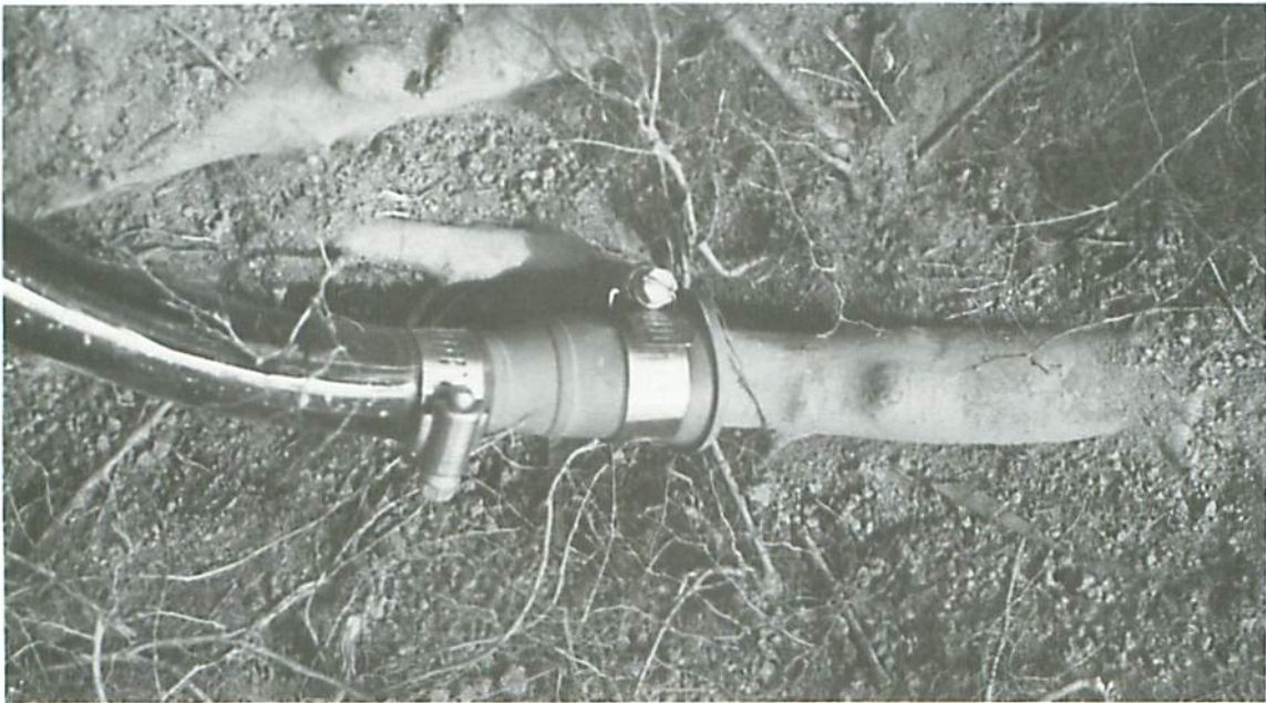
Fig. 4. Variable rubber adapter attached to a severed root.
