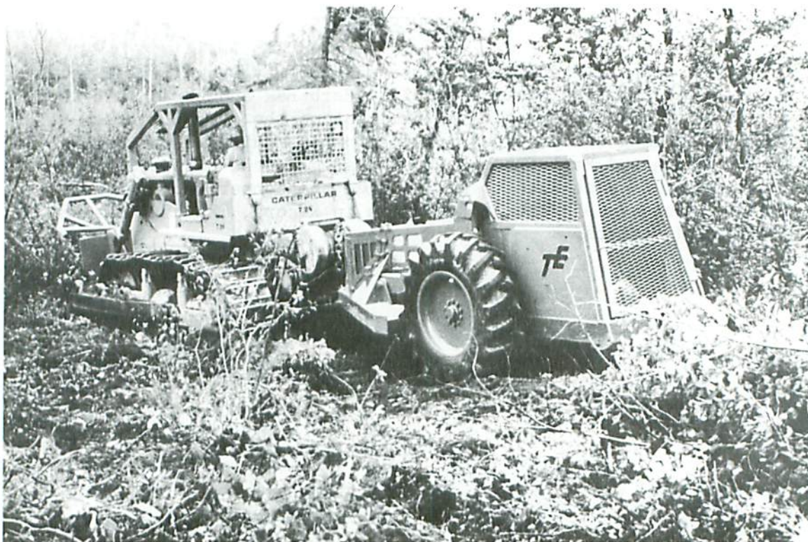
Frontispiece. The complete planting unit: Timberland Plow, Caterpillar D7E Bulldozer, and Timberland Planter.
