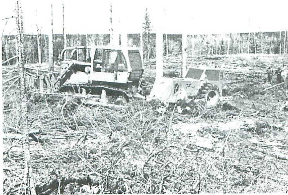
Figure 1. Vermilion Bay clay site. Timberland Plow, D7F Bulldozer, and Timberland Tree Planter weave through poplar residuals in southern corner of planting area.
