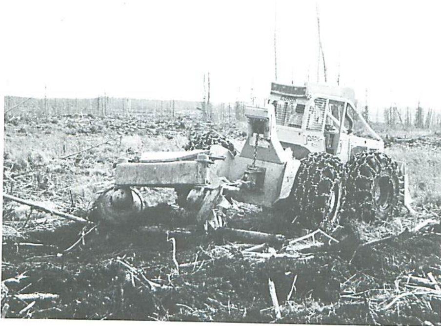
Figure 6. TTS Disc Trencher
