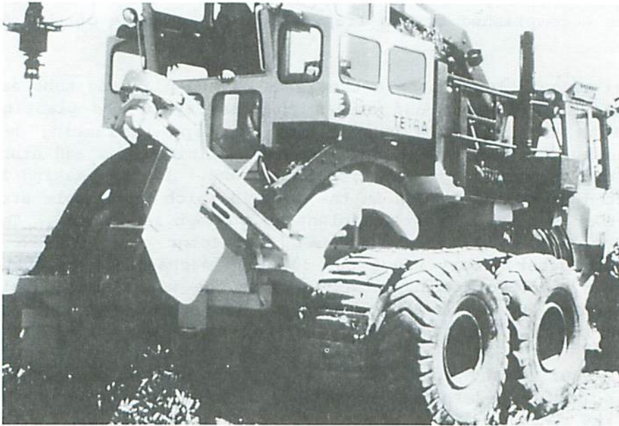
Figure 9. Planting mechanism on guide bars.
