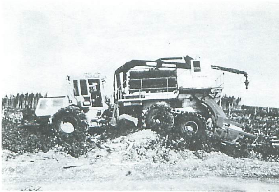
Figure 4. Tetra multifunctional semi-automatic tree planter mounted on a Bombardier BT-12 forwarder.
