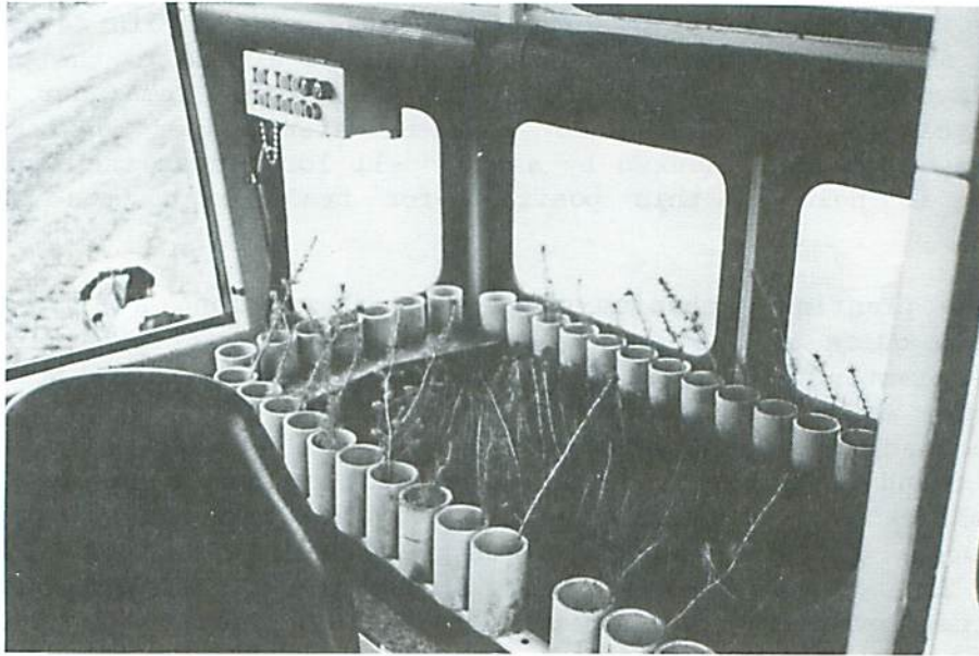
Figure 8. Rotating feed carousels in cab.
