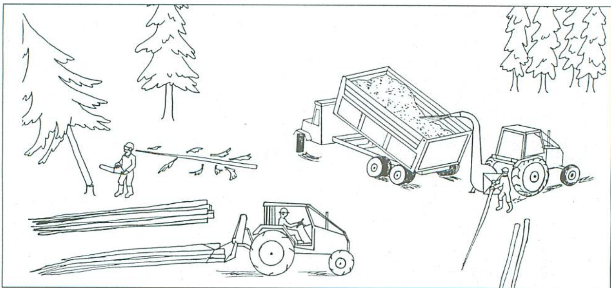
Figure 1. Option II: 4WD Tractor and chipping at the landing. (Illustration by K. McCallum)
