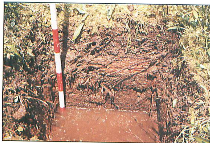
Figure 47. Profile of organic soil, showing fibric peat and a high water table; the range pole in the photo is marked in 10-cm segments (K. Baldwin).
