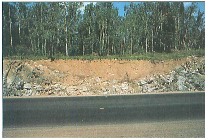
Figure 20. The depth of shallow soils typically varies over short distances as a result of undulations in the bedrock (G. Wickware).
