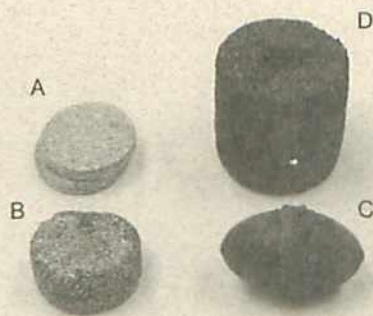
Figure 5. Examples of encapsulated seeds: (A) original FMC (single seed in a semispherical cavity of a flat, round disk formed by cementing together two identical halves of compressed vermiculite), (B) University of Idaho seed wafer (composed of seeds embedded in a tablet of a fine grade of vermiculite and activated charcoal, bound by methylcellulose), (C) Dupont "tree egg" (a blend of hydrophillic polymers, dried and pressed into a two gram, egg-shaped pellet into which the desired number of seeds is embedded), and (D) a fully imbibed Jiffy Products (N.B.) Ltd. J-9 wafer (compressed peat that has been bitumized to hold the wafer together following saturation and expansion).
