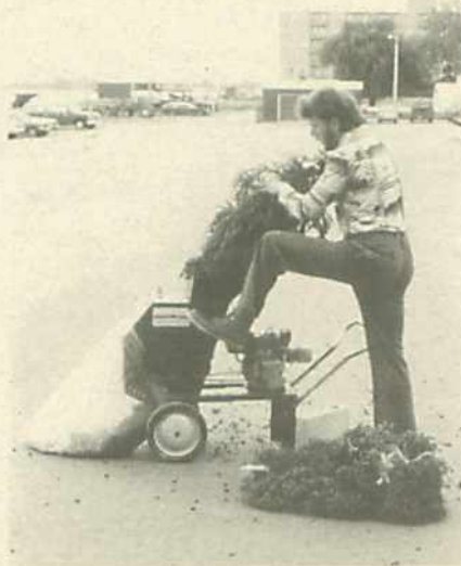
Figure 2. Hammer-mill type peat/soil shredder used to separate black spruce cones from branches.
