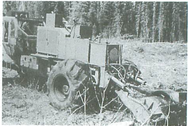
Figure 4013.1. The prototype one-row rototiller, powered by an auxiliary motor and mounted on a forwarder.
