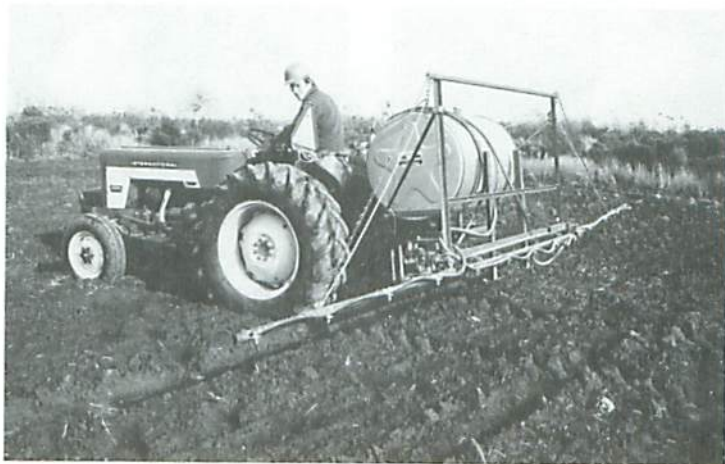
Herbicide spraying with a tractor-mounted sprayer with long boom.
