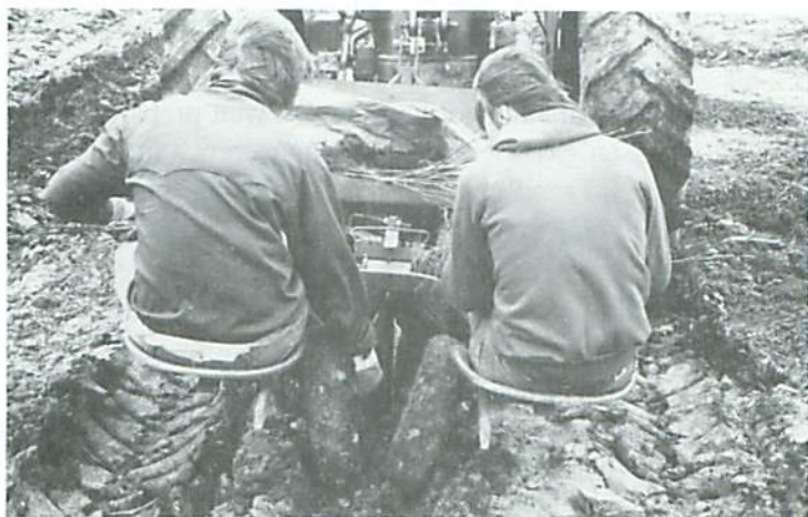
Rear view of the same planting machine. Note the unobstructed passage behind the packing wheel, which allows planting of tall seedlings.
