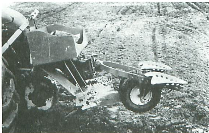
Side view of a small planting machine with a three-point hitch, suitable for pulling with a small farm tractor.
