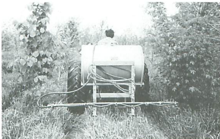
The same sprayer with a short boom to allow spraying between rows of trees.
